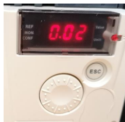
0.01 is corresponding to 1 hour of use. fig. 30. Display of use time for 230V single phased machine
